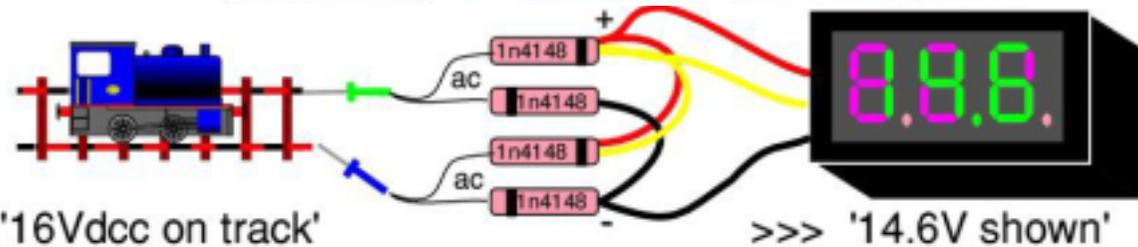
Common dcc 'on track' voltages are 14-16Vac for (00/H0) and 18-22V for G when measured from 0 to Peak (0-pk).
