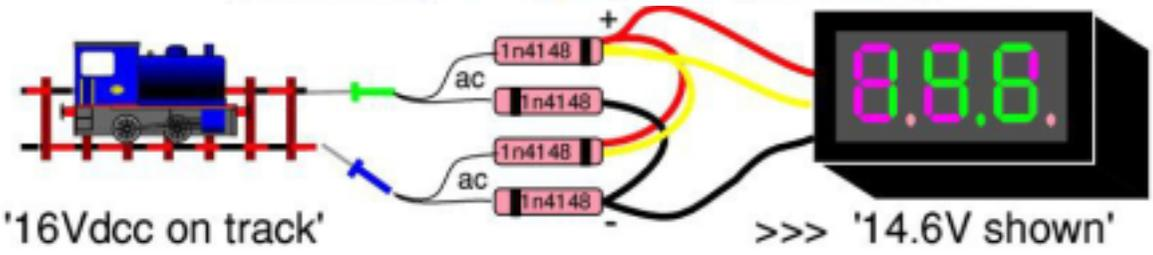
Common dcc 'on track' voltages are 14-16Vac for (00/H0) and 18-22V for G when measured from 0 to Peak (0-pk).
