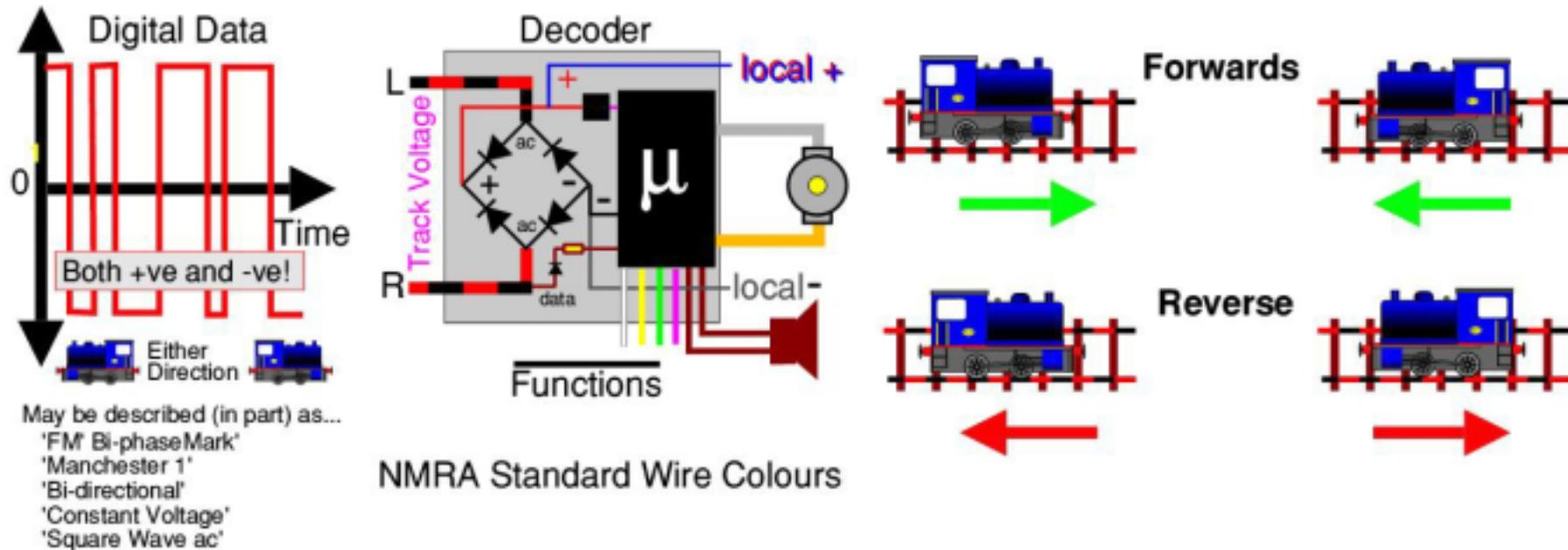
2-Rail Digital uses a 'constant amplitude' alternated onto the track at  $\sim 8.6\text{kHz}$ , by data transmitted from the Central Controller'. Hence it is an a.c. waveform albeit not a 'sinewave'! Half the signal would be blocked by a diode!
