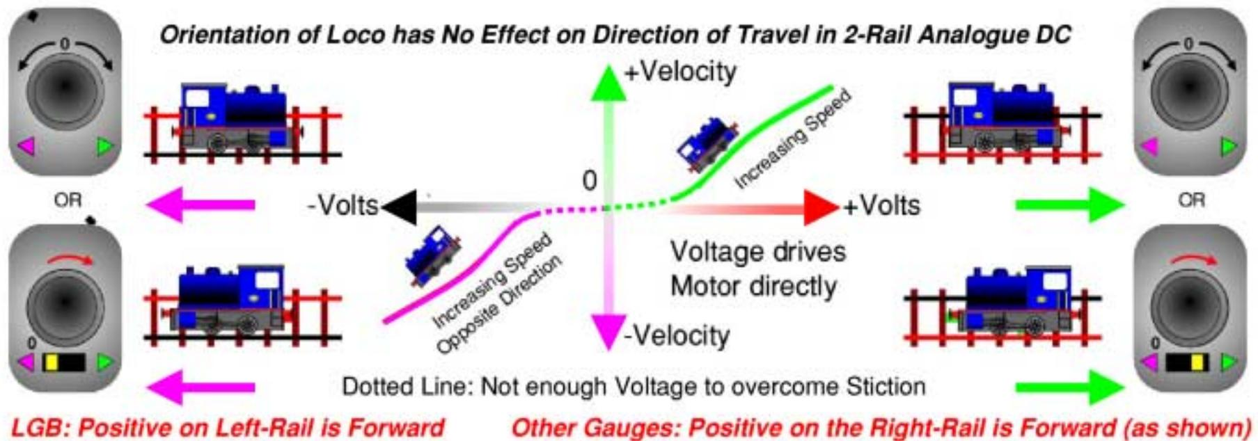
In the 'Traditional'/ Historical Method of DC Analogue Control shown above, a variable d.c. voltage is applied to the track.
