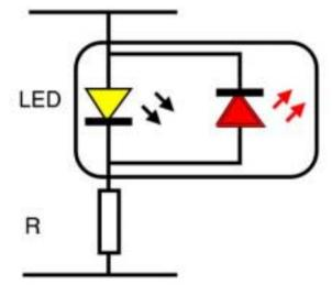
Compact 2-wire connection - but NOT really comptible with DCC ALTHOUGH they could be used in parallel to the 'Motor' outputs : However, they would go out when the loco stopped. This situation ALSO occurs in some pre-fitted models with LEDs
