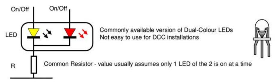
Common Anode (Positive) - 3-wire Bi-directional Lighting in Different Colours e.g. Red /White
