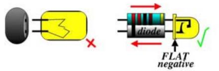
A Resistor to limit the current to 20mA or less A Diode for Protection An LED for the Light (Any Colour)
