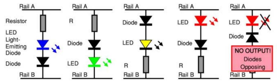
EACH of the different circuits shown, except the last, will light the LED when 'Rail A' is +ve compared to 'Rail B' -ve. In EACH case, the order of components is NOT important - ONLY the ORIENTATION of the Non-Linear Devices (Resistors, pieces of wire, light bulbs, switches etc are LINEAR and will work 'either way round')
