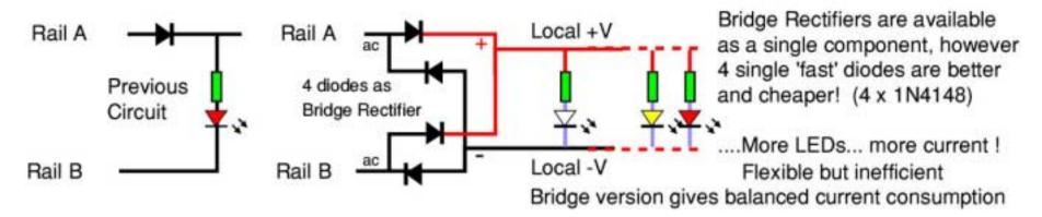
Adjust each individual resistor, as required, to adjust individual LED brightness - ideally suited to mixed colours. For analogue use, this circuit also brings the lights on at the lowest possible track voltage (3-6V according to colour) Typically, each LED and resistor will add another 5 - 10 - 20mA of load onto the output and also onto the track.
