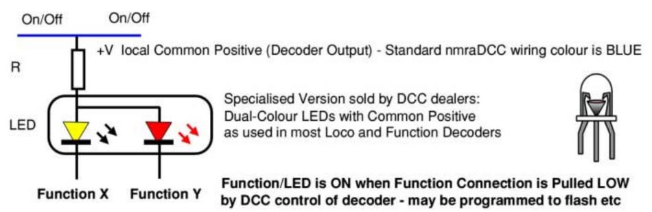
Universal Coach Lighting - ON ALWAYS for both DCC and DC track power (*Given enough Voltage!*) Modifying the left-circuit to 'Full Wave Rectify' the incoming dcc/dc track voltage (which is what Decoders do).....
