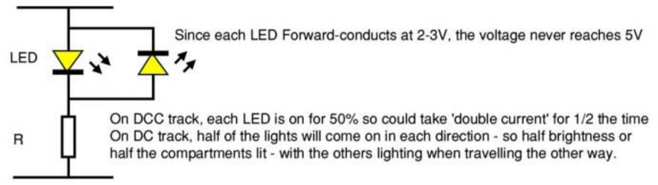
**Back to Front / Inverse Parallel LEDs - Bi-directional Lighting in Different Colours e.g. Red / White** Some Manufacturers offer 2-colour LEDs in one package, using just 2 leads - these conduct in opposite directions.
